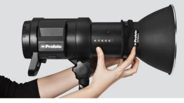
2 Before closing the clasp, adjust the light spread by sliding the reflector back and forth on the head.
